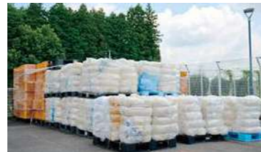
The company utilizes waste plastics, such as vinyl and film from the factory, as recycled fuel for thermal power generation.
